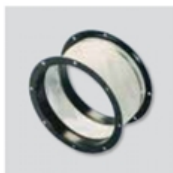
JBS/JBS-V Flat roof up stand - For mounting a fan on a flat roof without up stands. - For use on horizontal roofs. - Internal insulation to prevent condensation. - Supplied with screws and gasket for a complete weather seal.
