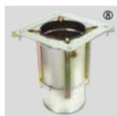
JBS Flat roof up stand - For mounting a fan on a flat roof without up stands. - For use on horizontal roofs. - Internal insulation to prevent condensation. - Supplied with screws and gasket for a complete weather seal.
