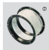
JBR N Flange - For use when circular connection is required directly to the fan. - To be mounted at the fan inlet with the JPA plate or fixed directly to the fan base (rivets or screws not supplied).
